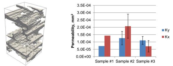
Figure 1: A voxel model of a unit cell in the non-crimp carbon preform (left); and the predicted permeability values for the three studied samples (right).
